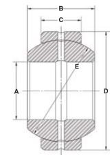
Standard - Spherical Plain - High Misalignment Bushings (Metric)
