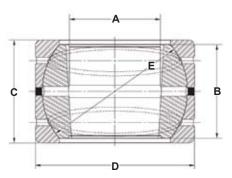
Spherical Plain - Double Acting - Extended Inner Ring - Outer Sleeve Bushing with Shim Pack
